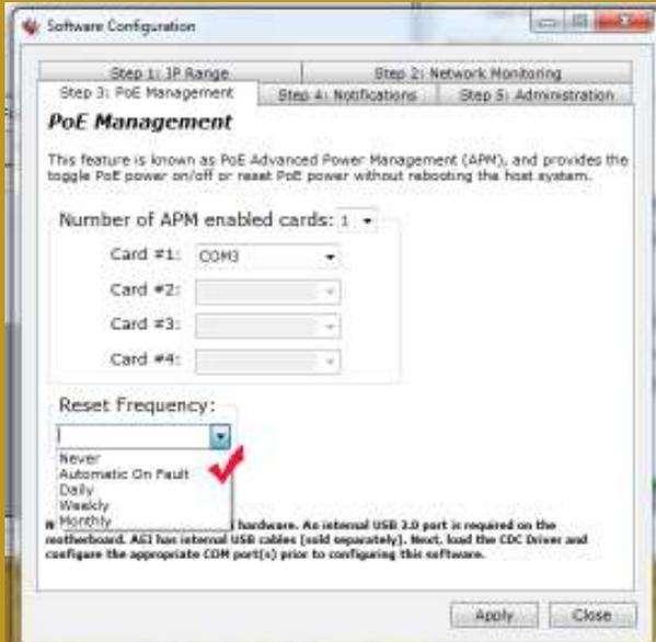
As can be seen above, the utility also can be configured to reboot PoE devices periodically for every 24 hours of continuous operation, weekly, or monthly.
